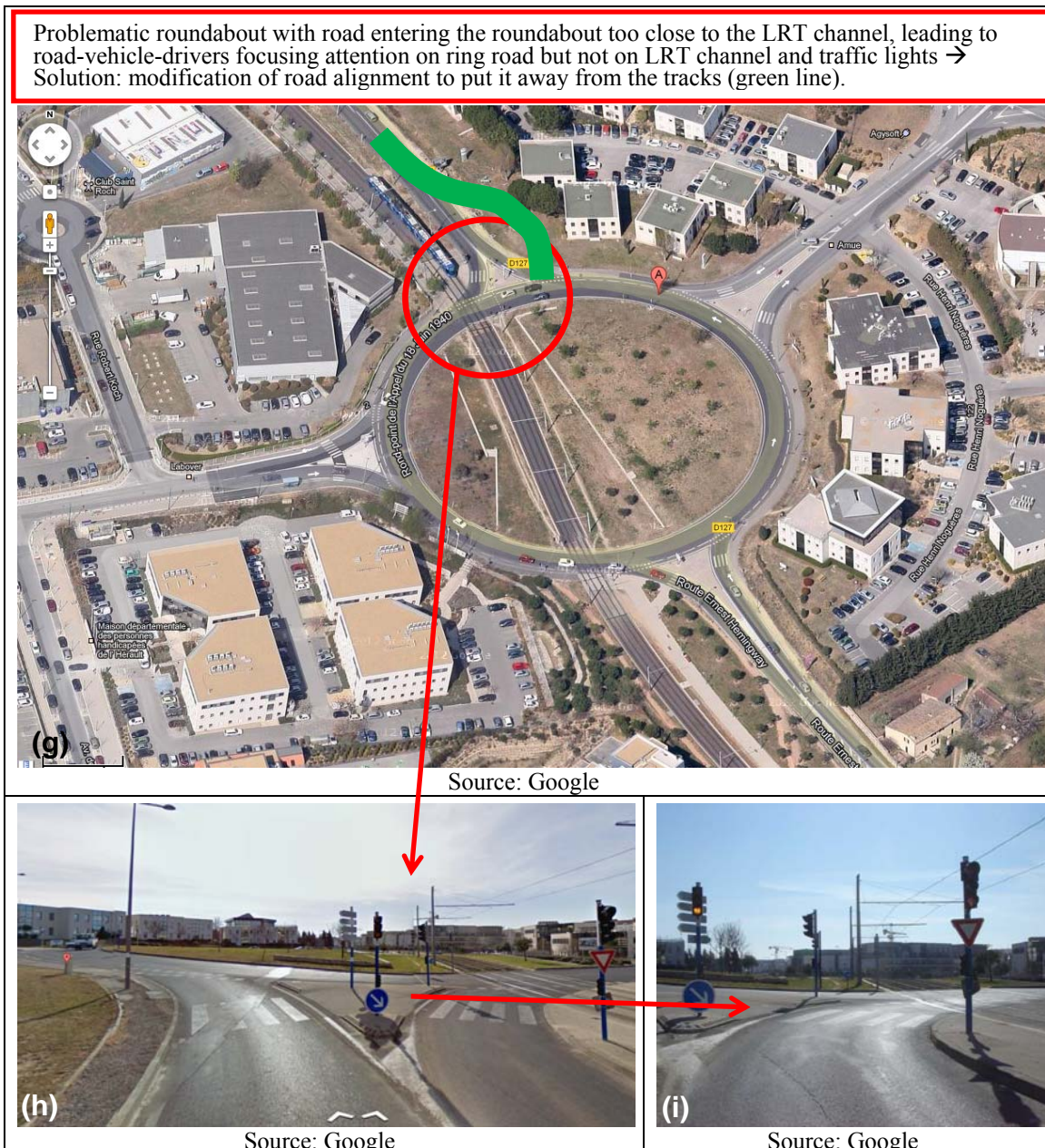
FIGURE 6 Roundabouts. a) Low vegetation in a LRT roundabout in Tenerife; b) Traffic lights for different approaching directions in Tenerife; c) Double small traffic lights for improving awareness in Tenerife; d,e&f) Modification of traffic lights operation for improving roundabout safety in Barcelona; g,h&i) Modification of the road layout for improving roundabout safety in Montpellier.
