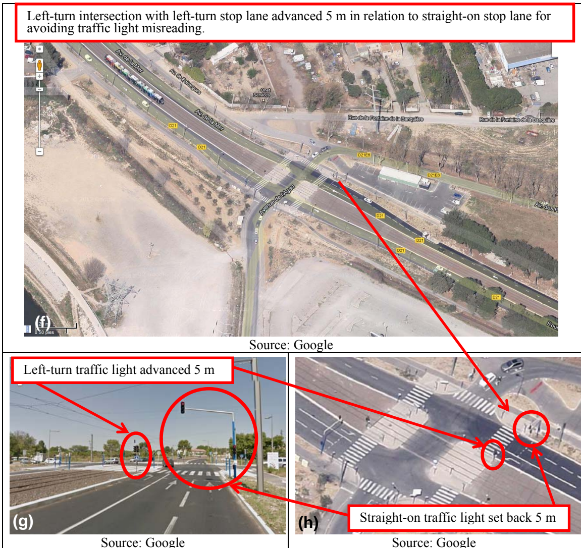
FIGURE 5 Left-turn intersections. a) Transforming a left-turn intersection into another kind of maneuver; b&c) Transforming a left-turn into a perpendicular intersection in Porto; d&e) Avoiding forbidden left-turns by means of bollards in Barcelona; f,g&h) Improving traffic lights readability in Montpellier.
