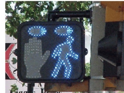
Illustration 26 : Signal « yeux animés » aux USA. (source : Federal Highway Administration, US Department of Transportation)
