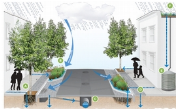
(A) street trees with flow through planters (B) rain gardens (C) upgraded sewer pipes (D) permeable pavement (E) cisterns (F) vegetated roofs
