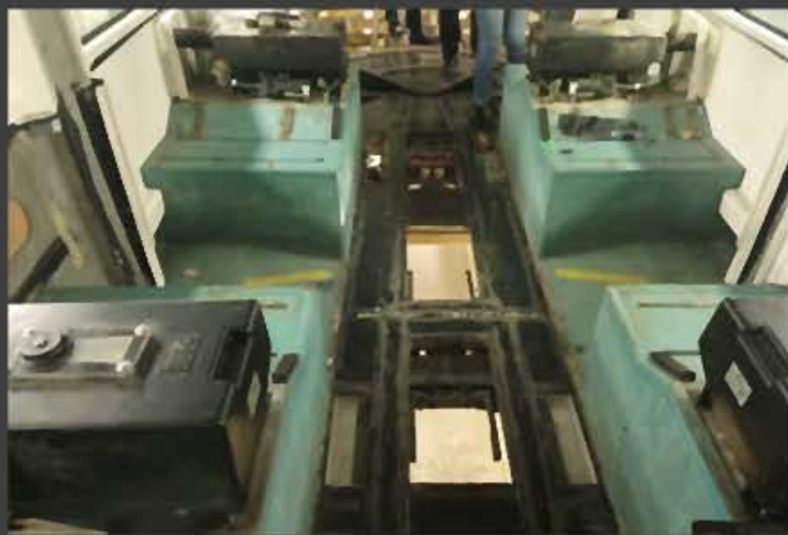
16 PAIRS OF SEATS BACK-TO-BACK WITH POWER ELECTRONICS BETWEEN, OVER MOTOR BOGIE
