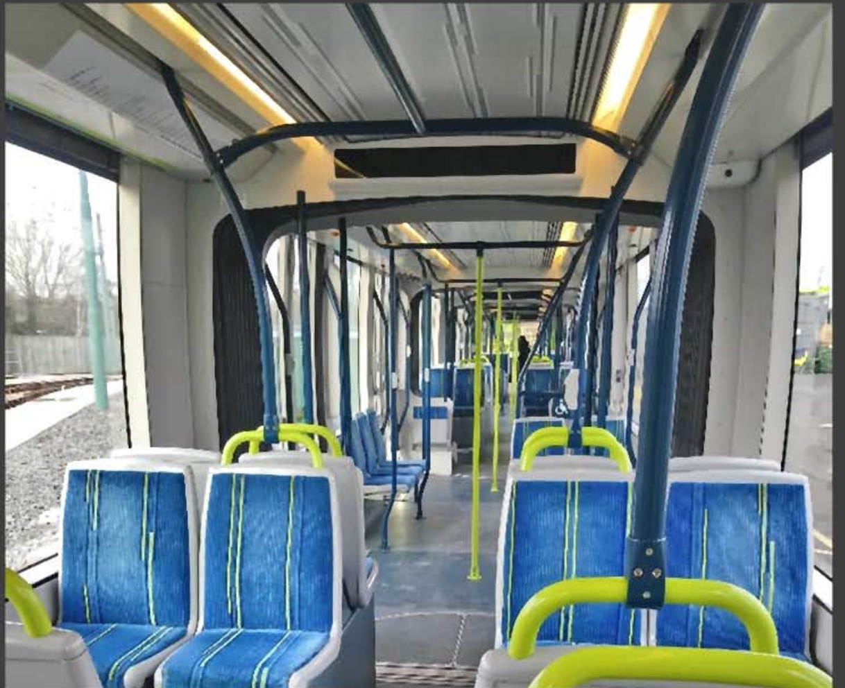
16 PAIRS OF SEATS BACK-TO-BACK WITH POWER ELECTRONICS BETWEEN, OVER MOTOR BOGIE
