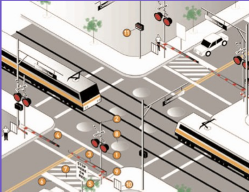
Four Quadrant Gates, typically located in Cab Signal Segment
