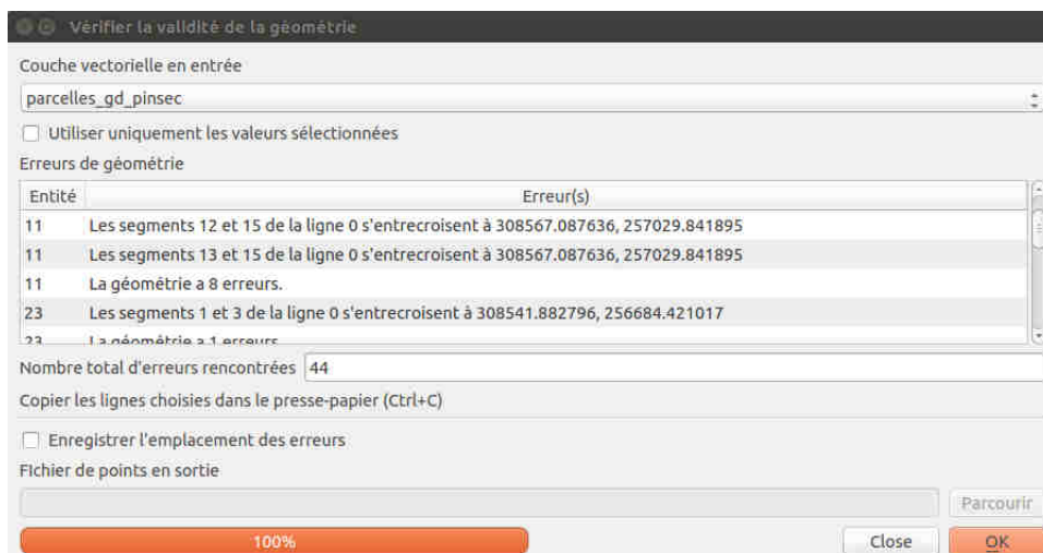
Figure A.1 – Error message given by Geometry validity of QGIS for parcel layer.
