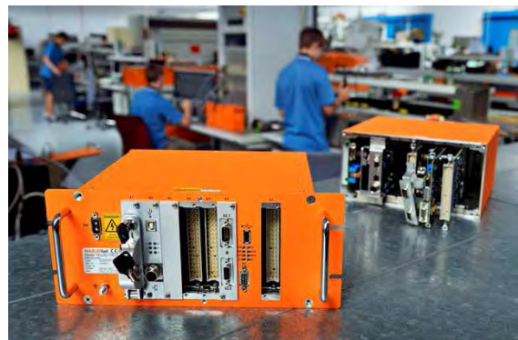
Figure 14 – Example of the commercially available black boxes - Black box type Teloc 1500 from Hasler Rail AG [Source: www.bernerzeitung.ch/region/bern/Dieser-Spion-faehrt-in-vielen-Zuegen-mit/story/24960723 ]
