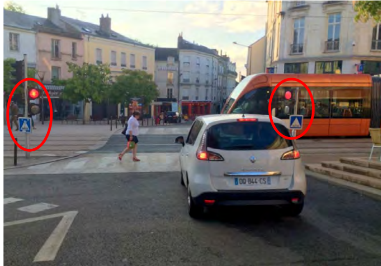
Figure 79 – Le Mans, Intersection Roosevelt – National, additional flashing traffic signals
