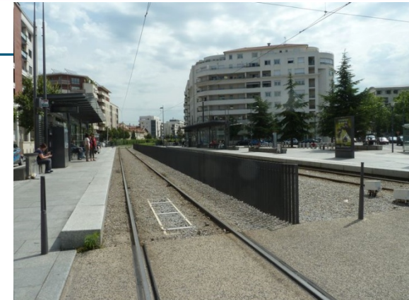
Lyon: example of barriers for configuration with lateral track/ dedicated platform/ separated traffic
