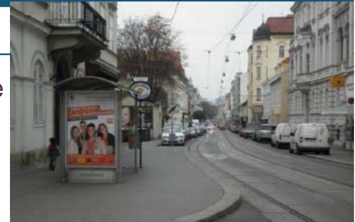
Wien: a platform cape for configuration with lateral track/ dedicated platform/ mixed traffic
