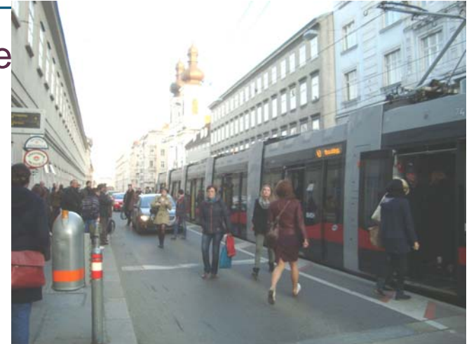
Wien: example of configuration with central track/ no dedicated platform/ mixed traffic
