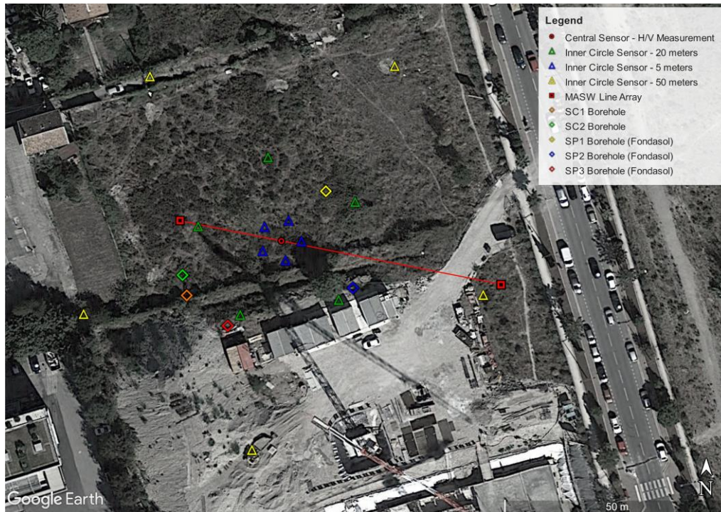
Figure 7. Position of the stations of the seismic array (triangles) and the MASW profile. Boreholes SC1 and SC2, where accelerometers will be installed, are shown by orange and green diamonds. Geotechnical boreholes SP1, SP2 and SP3 by yellow, blue and red diamonds
