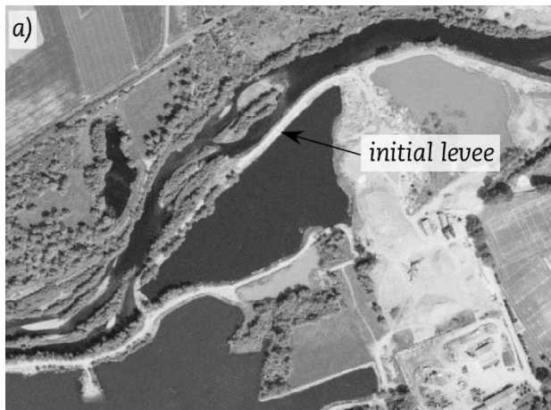
Gravel pit of “Pont Lamothe” (Lamothe, France) : a) in 1992 and b) in 1995. The 1994 flood of the Allier river has caused the river capture by the gravel pit.
