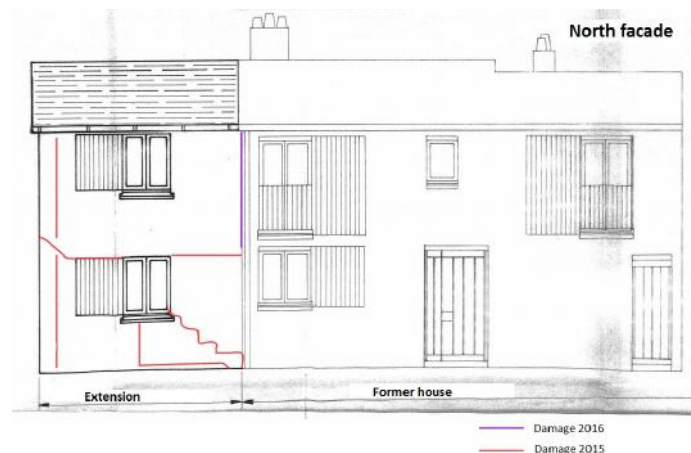
Figure 3: Noticed damage survey in 2015 and 2016
