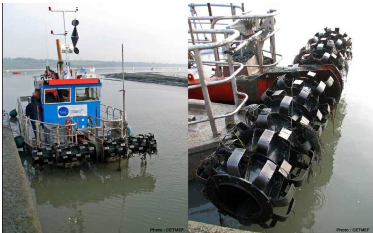
Figure 2-4: Rotary milling cutter dredger Le Rochevilaine used in the Vilaine estuary (source: CETMEF)
