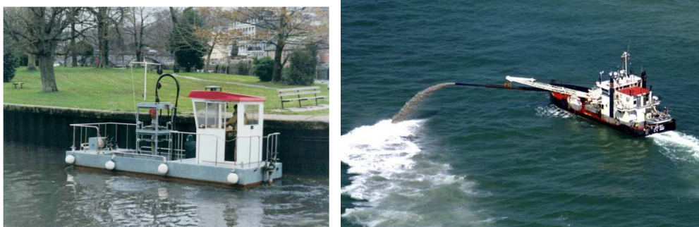
Figure 2-1: The agitation dredger Neptune (source: terra et aqua ), and the dredger Side Cast Merrit (US Army Corps of Engineers)
