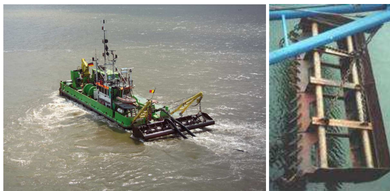
Figure 2-3: The plough dredger Alligator (DEME) and detailed view of a leveller (source Anthony Bates Partnership)
