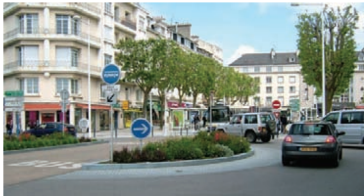
Lorient : a lot of small traversed roundabouts in the central section where all speeds are limited to 30 km/h; there are no traffic lights due to the irregular bus flow (up to 8 lines)
