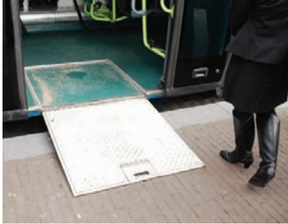
Manual ramp: observed in all BHLS schemes in Sweden, Netherlands, Germany; suitable due to a very low use throughout the day, even into the bi-articulated bus of Hamburg; handled by the drivers.
