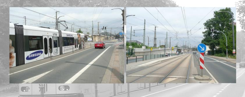
Dresden: Standard platform in one direction – trafficable platform in the other (with traffic signal for car traffic)
