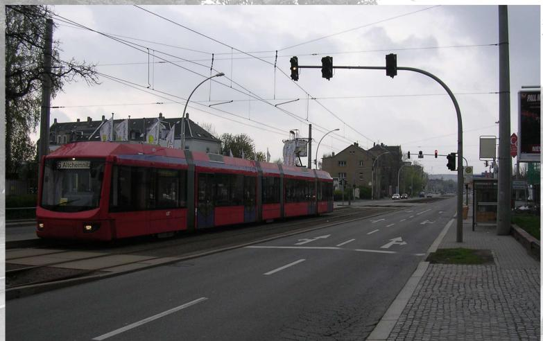
Picture shows an old style "street stop" which does not fulfil todays level access requirements. Trafficable platforms are to be seen as an upgrade to these stop types.
