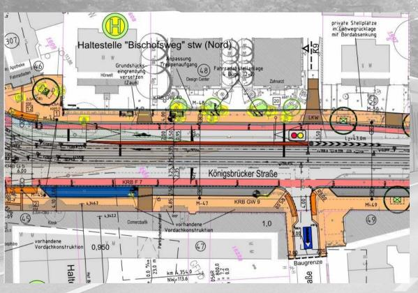
Dresden: trafficable platform in a location with two parallel car lanes (with traffic signal for car traffic)
