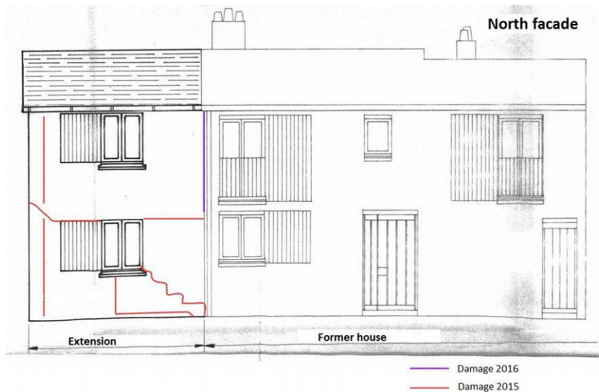
Illustration 44: Noticed damage survey in 2015 and 2016
