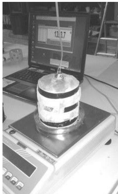
Illustration 9: Calibrating a soil sample in laboratory
