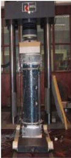
Figure 2. Cyclic displacement imposed on CFRP strengthened column (UNL) and axial tests on confined cylinders (IST)
